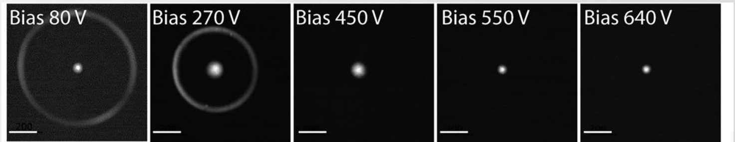
Standard Truncated LaB 6 filament
